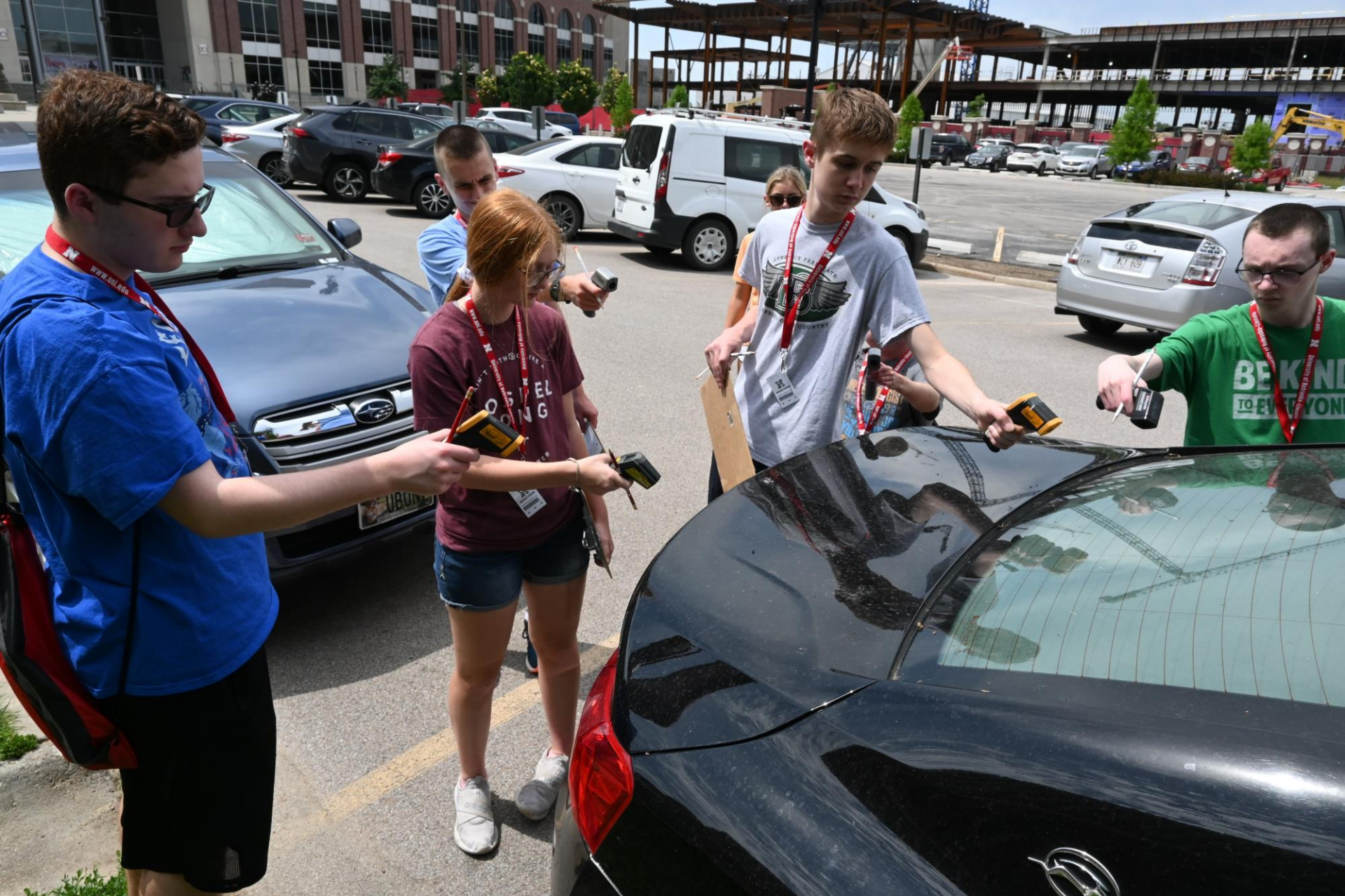
Comparing the surface temperatures of various colors of cars in a parking lot
