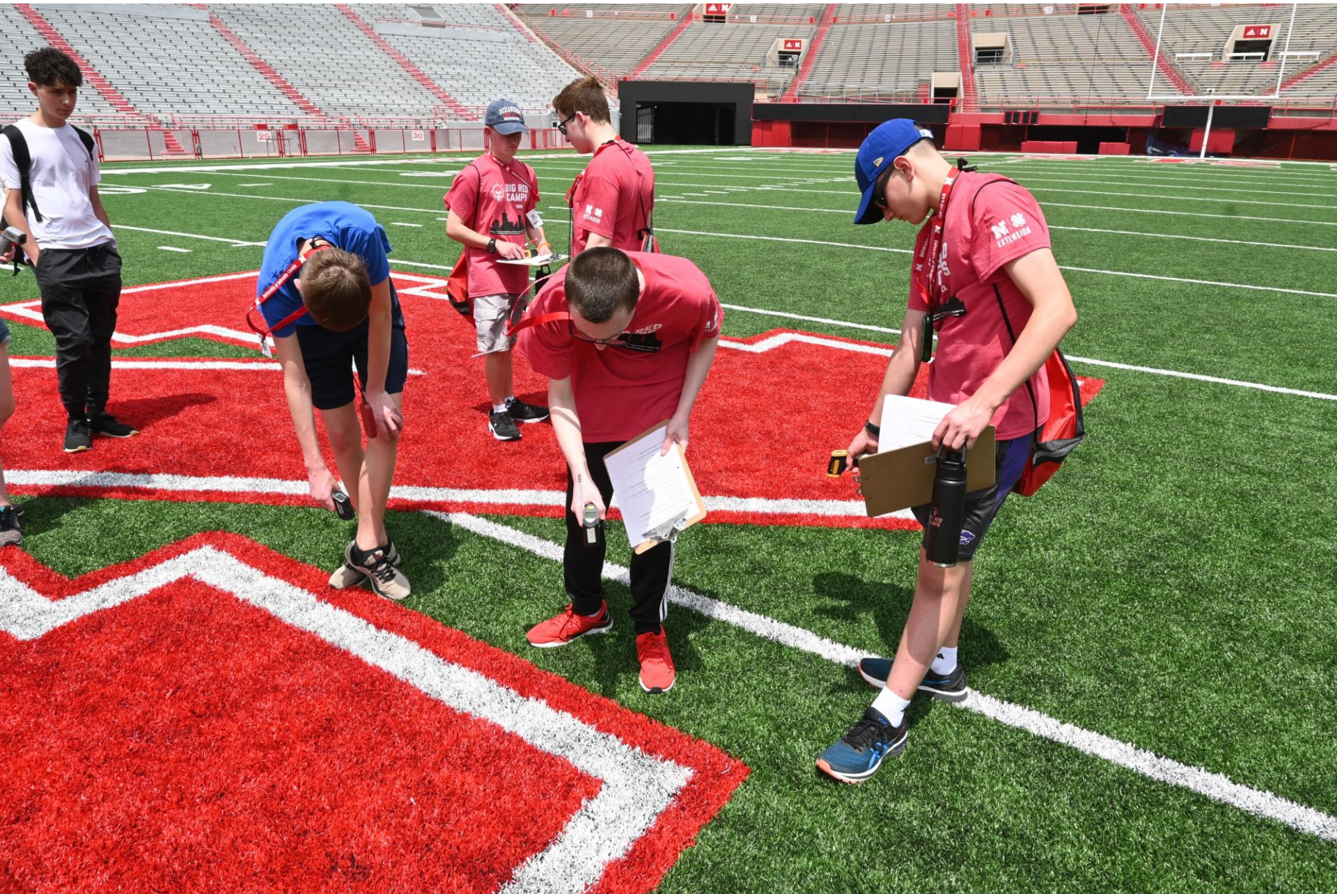
Measuring the temperatures of different colored surfaces on the Memorial Stadium field. We found temperatures as high as 137°F
