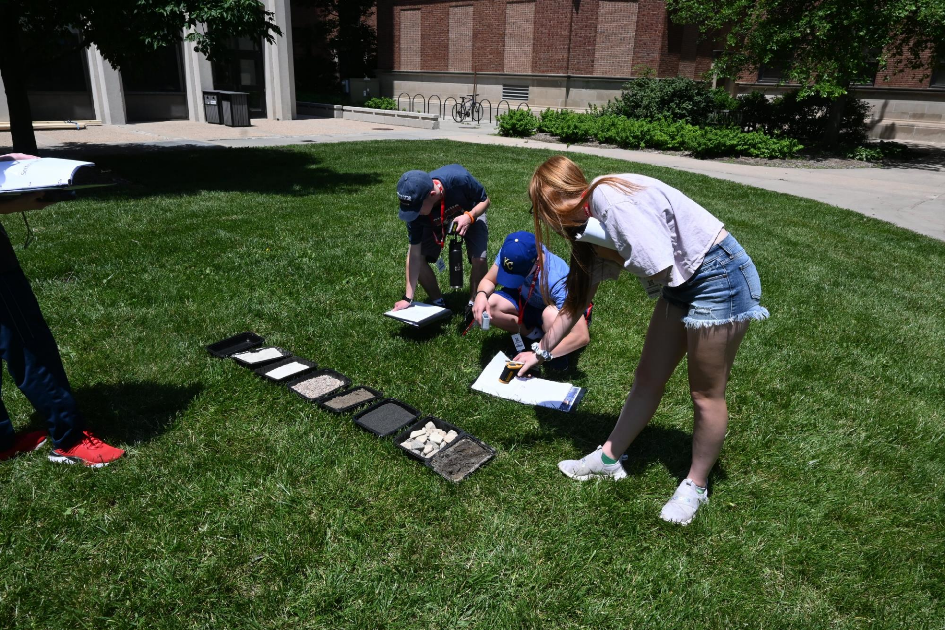
Conducting an experiment measuring the rate of warming of 8 different surface types in the sun: water; dry sand; wet sand; gravel; dry soil; black sand; large rocks; & wet soil
